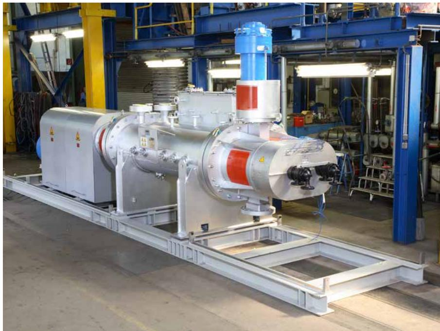
The versatile reactors are characterised by very large process volumes and excellent self-cleaning. The two co-rotating rotors of Reacom and the counter-rotating rotors of Reasil provide plug flow capabilities of products with a wide range of viscosities. The high degree of self-cleaning is achieved by the intermeshing of specially shaped rotor elements. The rotors and shells of both processors can be heated or cooled.
