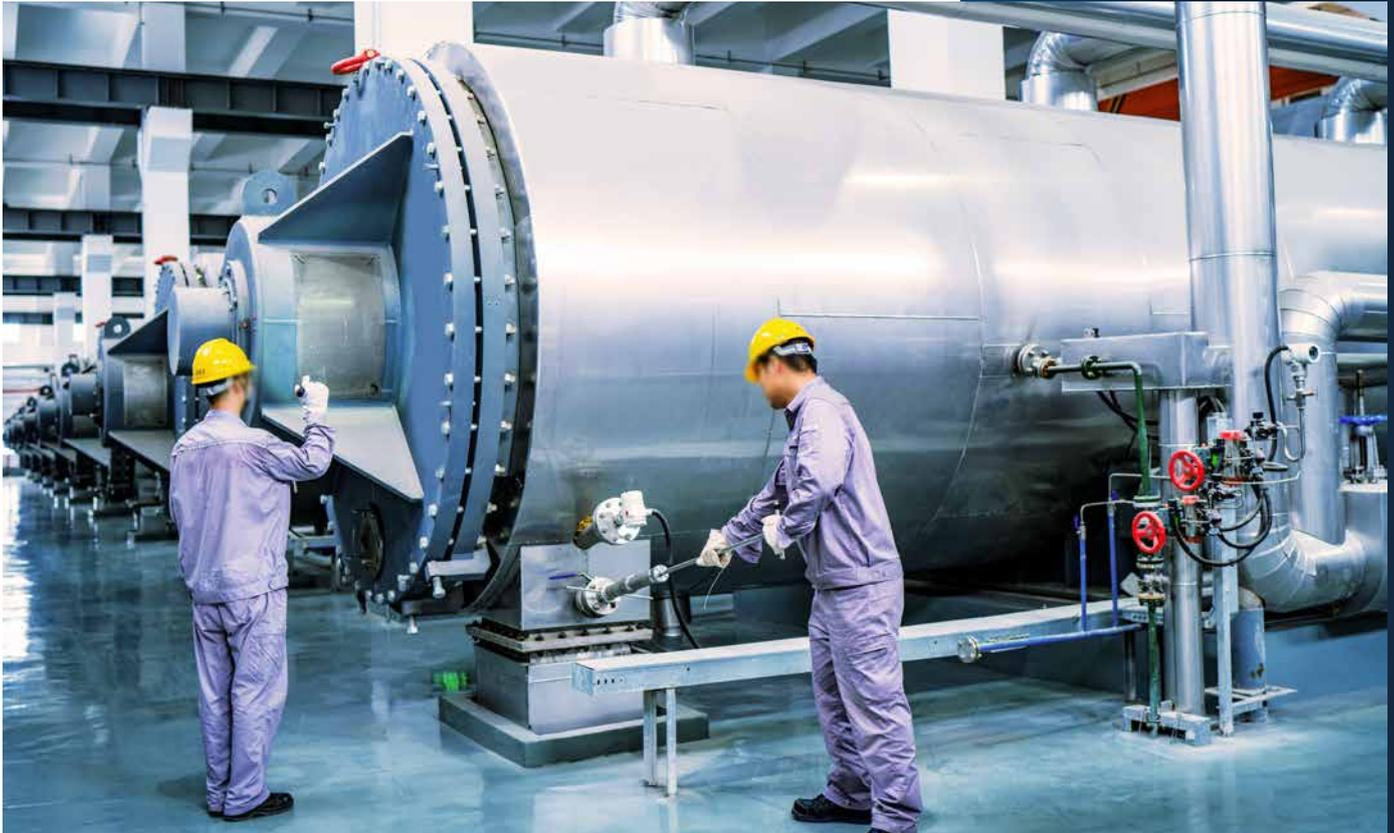
**This type of dryer is a continuously operating contact dryer, which offers the following unique advantages:**
